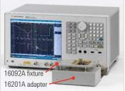
Impedance measurement with reflection method (for low-to-middle impedance)
