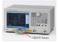
Impedance measurement with gainphase series-thru method (for middle-to-high impedance)
